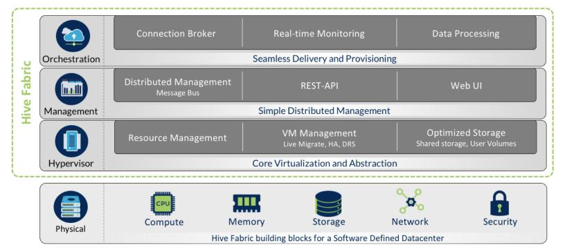
**Physical**: Hive Fabric is a simple bare metal install from ISO or PXE server supporting a wide range of x86 hardware. A cluster is quick to build and can start from a single server and scale to hundreds of servers and beyond as the solution is put into production.
